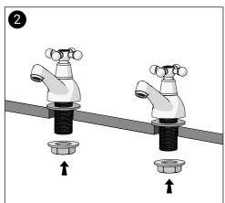
Whilst holding the tap in place, screw the back nut onto the tap tail and tighten. Do not over-tighten as this may damage the mounting surface.
