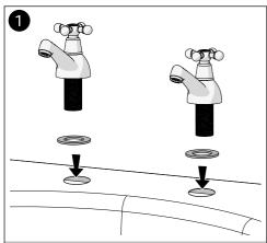
Ensure that all parts are present before installation. Install the taps onto the bath leaving the washer on the tap tail.
